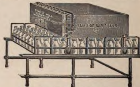
Fig. 247. Sanitary milk-bottle filler.
